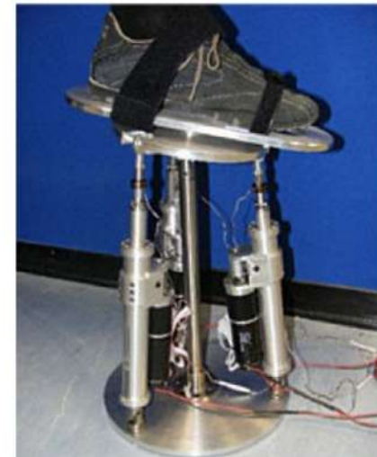
High Performance Ankle Rehabilitation Robot
